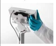
Place your terminal on a stand which is quickly mounted at the back of your balance. The display is easier to read and good posture is maintained.
