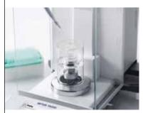
For routine pipette testing, an evaporation trap significantly reduces moisture loss of the test liquid and can be mounted on your balance in seconds.
