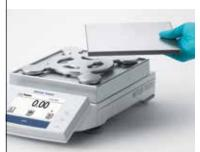
SmartPan makes your weighing and dosing processes more comfortable and convenient by enabling you to use your 1 mg balance without a draft shield.
