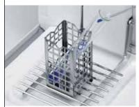
The Faraday cage effect of the ErgoClip basket protects the weighing cell from electrostatically charged samples and containers. Supplied as standard with all analytical balances.
