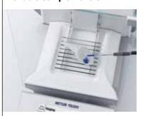
SmartPrep<sup>™</sup> single-use, antistatic funnels enable safe and fast weighing-in of powders. Simply weigh, transfer and rinse. Fits nearly any standard 5-250 mL flask.
