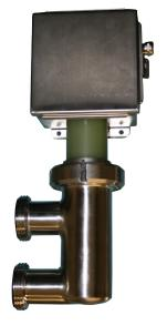
The product flows through the pipeline where the moisture measurement is taken. The Application Interface is made up of a pipe with attached sensor electronics that is integrated into the pipeline framework of the production process. An optional heater jacket ensures that the product does not solidify. Typically used with production processes manufacturing fluids, pastes, and confectionery applications.
