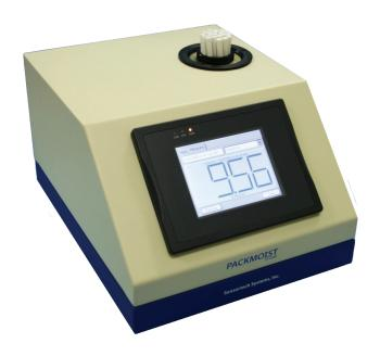
Prior to PACKMOIST's development the need to test cigarettes in their finished state of production had been accomplished through Near Infrared Reflectance (NIR) laboratory analyzers. This method of testing required manufacturers to carefully remove the tobacco from the cigarette casing and place the contents in its test bed. Providing a simple and non-destructive alternative to this messy and wasteful process was the objective behind PACKMOIST's innovative design.
