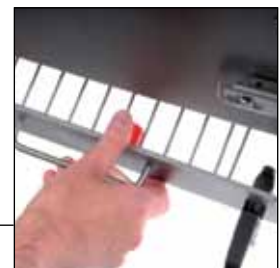
Integrated test facility provides efficient means of testing detector performance and reject diverter operation
