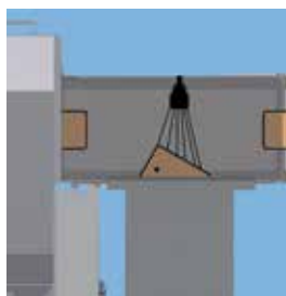
Air blast reject system
