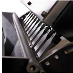
Air-blast reject system
