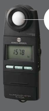
Receptor diffuser window: Ø **25** mm
