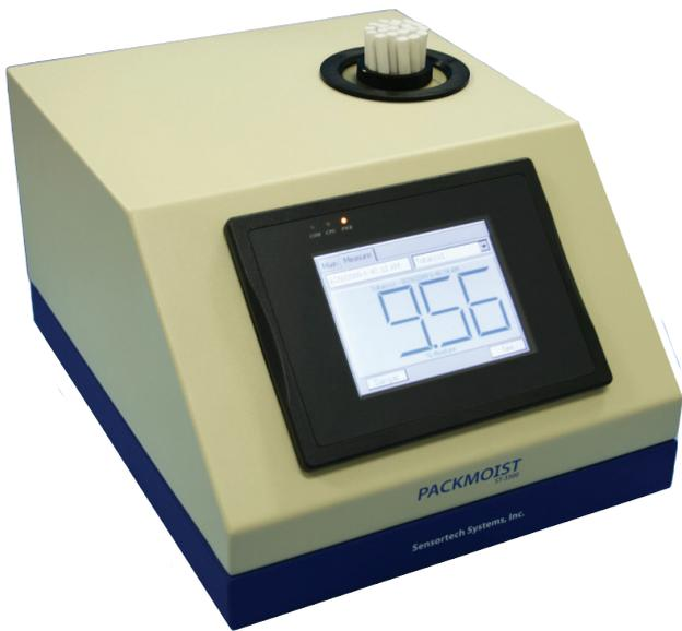
The PACKMOIST Laboratory Moisture Analyzer uses Radio Frequency Dielectric Technology to provide an accurate moisture measurement of 20 cigarettes in their finished state of production. Simply placing a complete pack of cigarettes in PACKMOIST's cylindrical test chamber provides an instant moisture measurement displayed on its Operator Interface.
