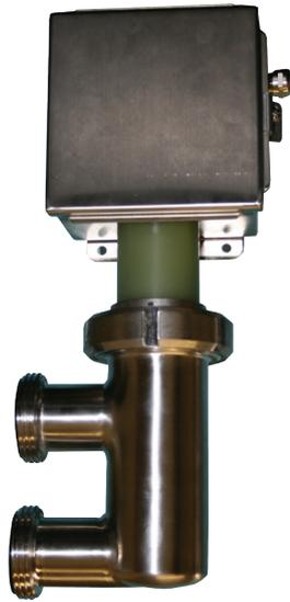
The product flows through the pipeline where the moisture measurement is taken. The Application Interface is made up of a pipe with attached sensor electronics that is integrated into the pipeline framework of the production process. An optional heater jacket ensures that the product does not solidify. Typically used with production processes manufacturing fluids, pastes, and confectionery applications.
