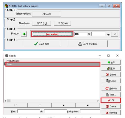
Provide cargo data by pressing "OK", select a load and confirm.
